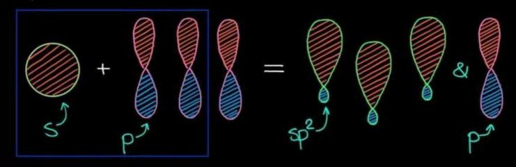
Sp<sup>2</sup>-hybridized orbitals form a trigonal planar shape
